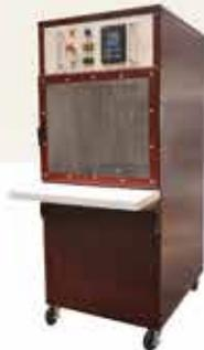
AC, 20 kV, ASTM D149
